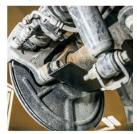
4. Ensure to make the two open tab holes sit against the caliper bolts before re-tightening the bolts to the factory specs.
