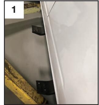
6. Once board is in place, mark on the running boards where the center bracket now lines up and where your new holes need to be drilled. You can alternatively drill pilot holes
