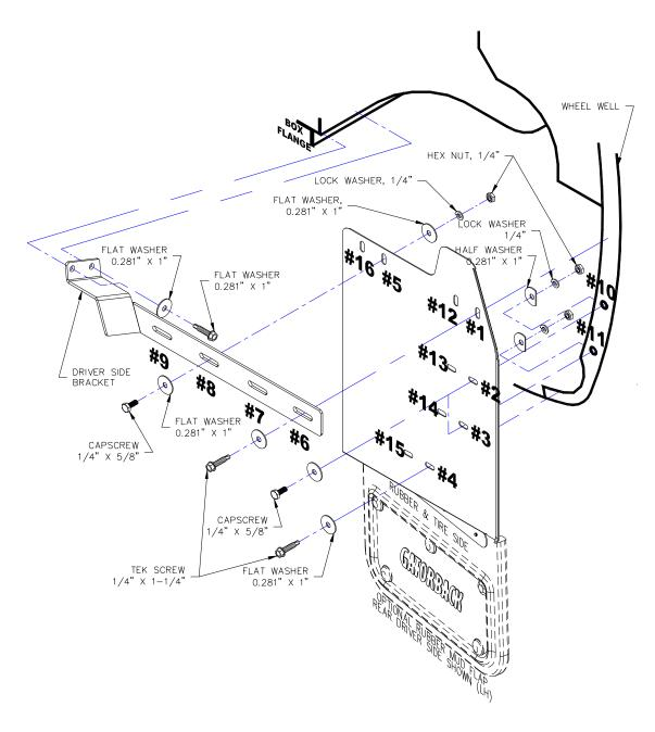
✓ Check all fasteners for tightness. Repeat procedure on the passenger side
