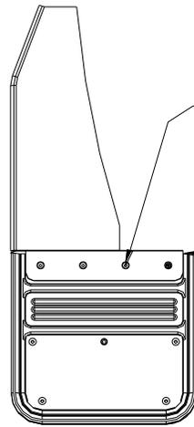
DRILL FOUR Ø3/16" HOLES FROM THE STAINLESS PANEL THROUGH THE RUBBER FLAP
