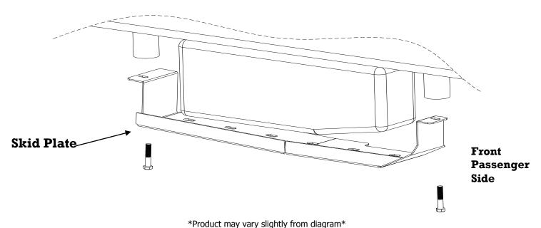
Installation: Remove factory cab mount bolts; place the skid plate over the Factory Urea Tank Cover. Reinstall factory bolts and tighten.
