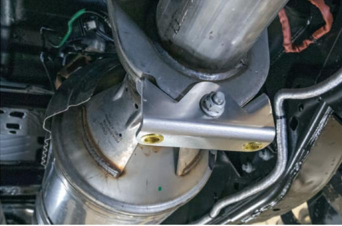
5. Secure guard to the bottom of the mount brackets shown here
