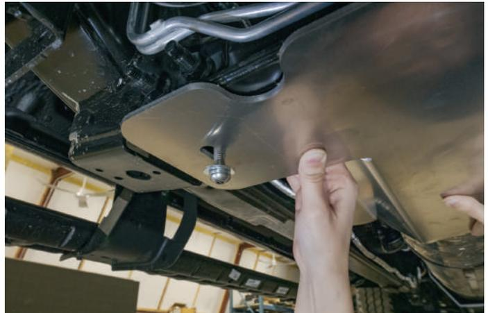
6. Loosely secure guard to the previously tapped hole with a flat washer (c), lock washer (d) & self threading screw (a)
