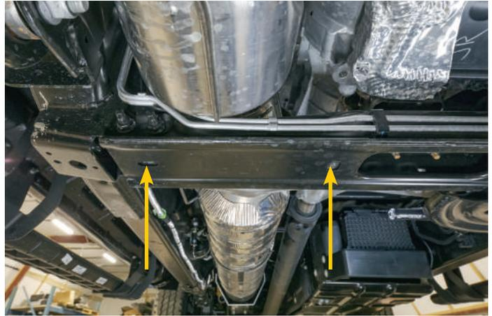
5. Loosely secure the front of the guard to the mount plate holes using 2x flat washers (c), 2x lockwashers (d), & 2x button head screws (b)
