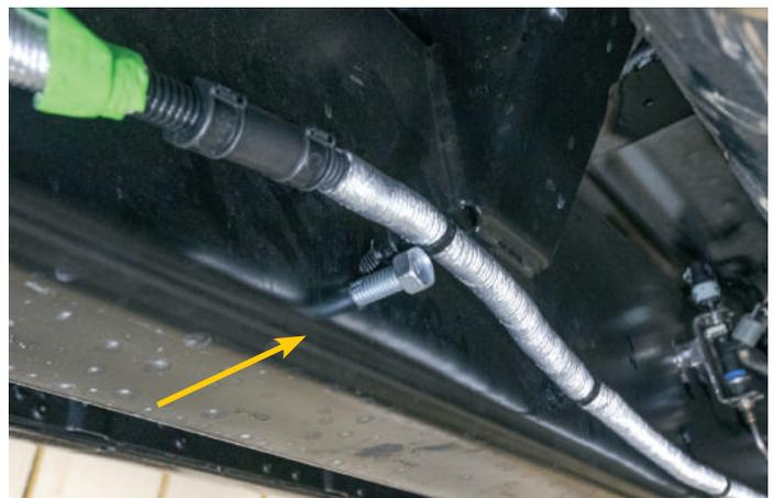
4. Insert the mount plate into the transmission mount access hole. Slide it in until the two mount holes align with factory holes in the cross member
