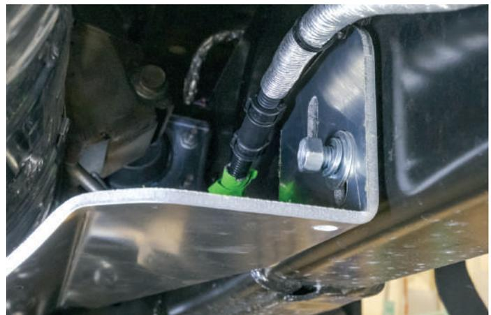
7. Check the alignment & tighten all fasteners
