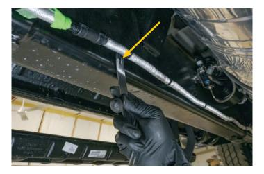
3. Use the supplied thread cutting screw to pre tap the existing hole where the cable clip was removed
