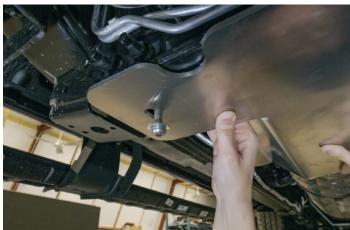
6. Loosely secure guard to the previously tapped hole with a flat washer (c), lock washer (d) & self threading screw (a) \*Please note: use left hole for 17-22 SD & hole on right for 23-C SD
