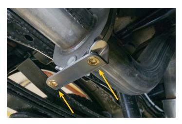
6. Secure Rear Guard to the brackets installed in Step 3 using 4 Flat Washers (b), 4 lock washers (c) & button head screws (a)
