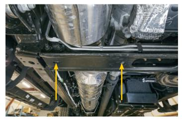
5. Loosely secure the front of the guard to the mount plate holes using 2x flat washers (c), 2x lockwashers (d), & 2x button head screws (b)
