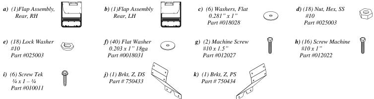
Prior to installation of your Mud Flap, see the above diagrams and parts list for all necessary parts. Start on the driver side.
