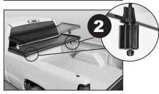
2. Secure cab clamp hooks under the metal bed rail.
