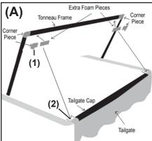
of foam and measure from the edge of the tailgate piece to the edge of the corner piece on both sides, cut and stick to existing foam.
