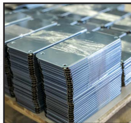
Bending complete and ready to stamp
