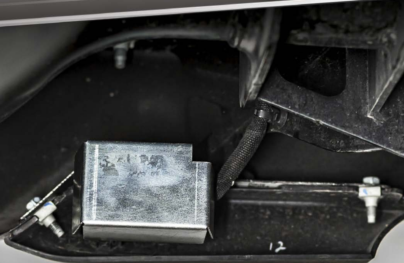
Backup Sensor Guard After P700366
