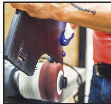
Burs are removed
