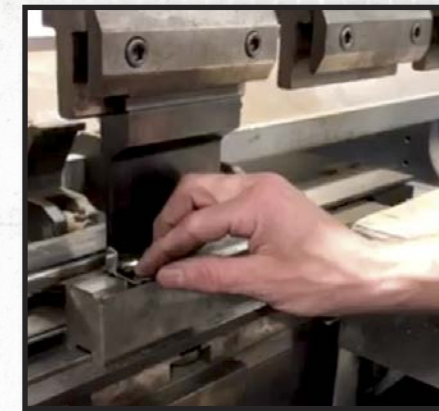
Custom fabricated clips bent by hand
