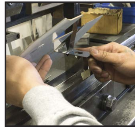
Hand bending a custom bracket
