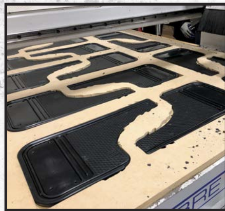
Mudflaps are routed in-house
