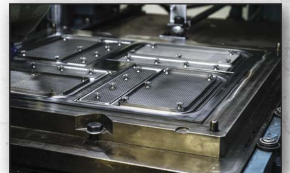
T-Nuts are embedded in the rubber
