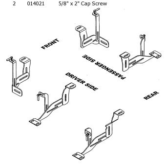
Note Orientation of Bracket Flanges and Braces. Use hand tools only!
