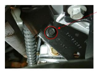
Remove M8 Factory Bolt from Shifter Linkage Bracket
