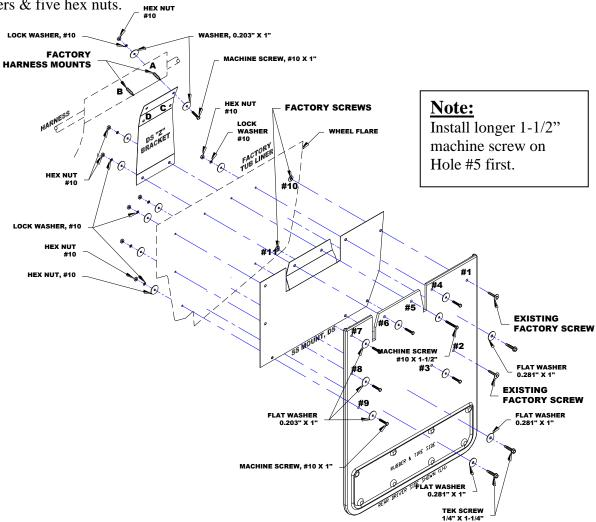
$\checkmark$  Check all fasteners for tightness. Repeat procedure on the passenger side
