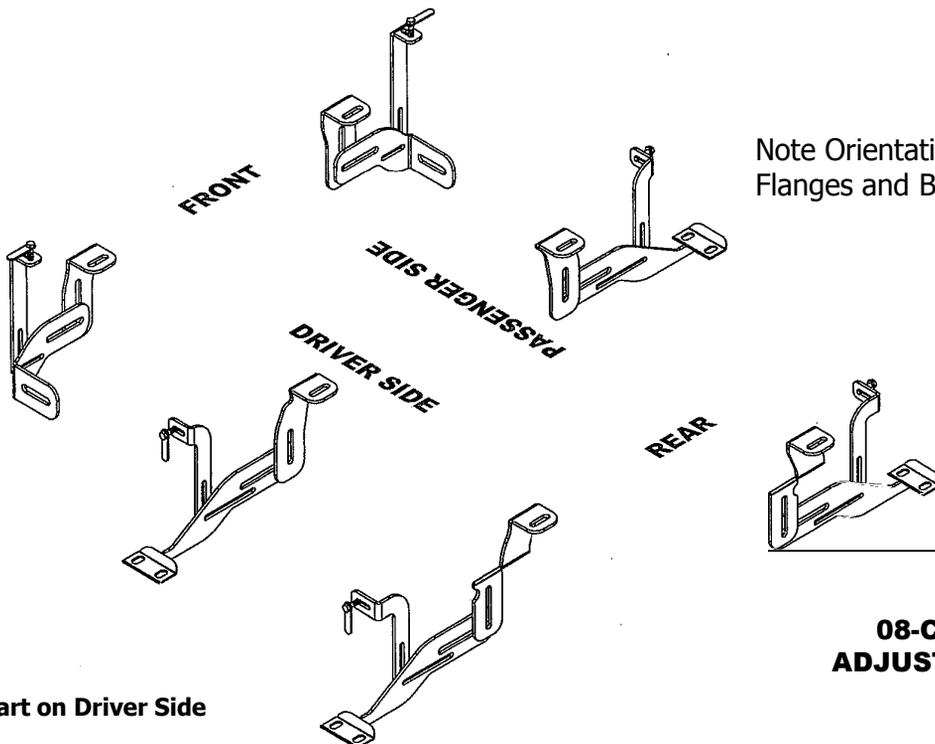
Note Orientation of Bracket Flanges and Braces
