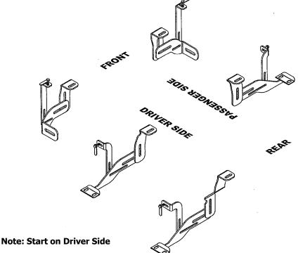
Note Orientation of Bracket Flanges and Braces
