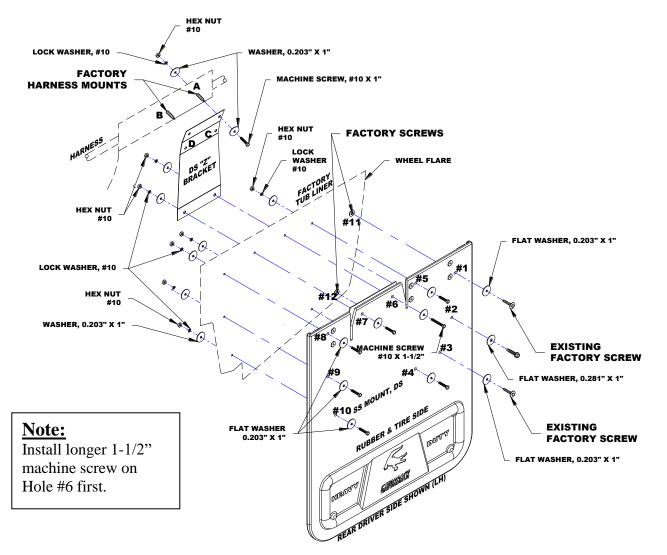
5. Drill a <sup>1</sup>/<sub>4</sub>" hole (7 places) from holes #4 to #10 through the factory tub liner then fasten holes #6 & #7 with two machine screws, the long screw used on holes #6, four flat washers, two lock washers and two hex nuts through the factory tub liners and Z bracket. For the remaining holes #4, #5, #8 to #10 with five machine screws, ten flat washers, five lock washers & five hex nuts through the factory tub liners.
