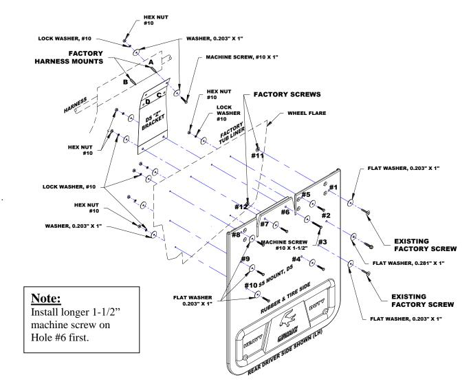
5. Drill a ½" hole (7 places) from holes #4 to #10 through the factory tub liner then fasten holes #6 & #7 with two machine screws, the long screw used on holes #6, four flat washers, two lock washers and two hex nuts through the factory tub liners and Z bracket. For the remaining holes #4, #5, #8 to #10 with five machine screws, ten flat washers, five lock washers & five hex nuts through the factory tub liners.
