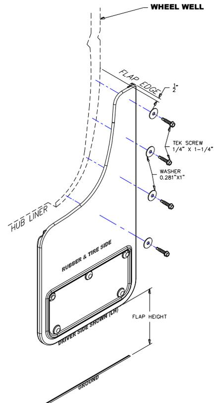
✓ Check all fasteners for tightness. Repeat procedure on the passenger side.
