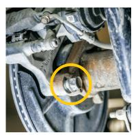
3. Position the guard in front of the train axle & slide the top open tab hole of the guard into the top caliper bolt. Swing the bottom open tab hole of the guard into the bottom caliper bolt. (\*Please note: it's important to install the top mount first).
