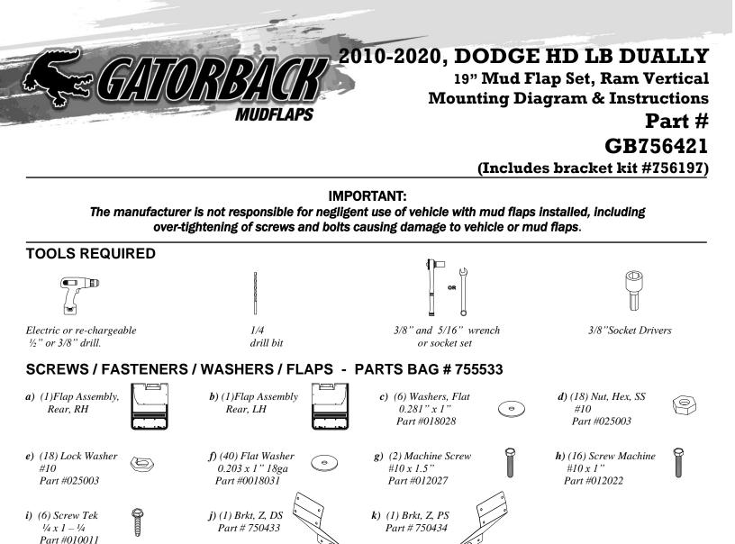
Prior to installation of your Mud Flap, see the above diagrams and parts list for all necessary parts. Start on the driver side.
