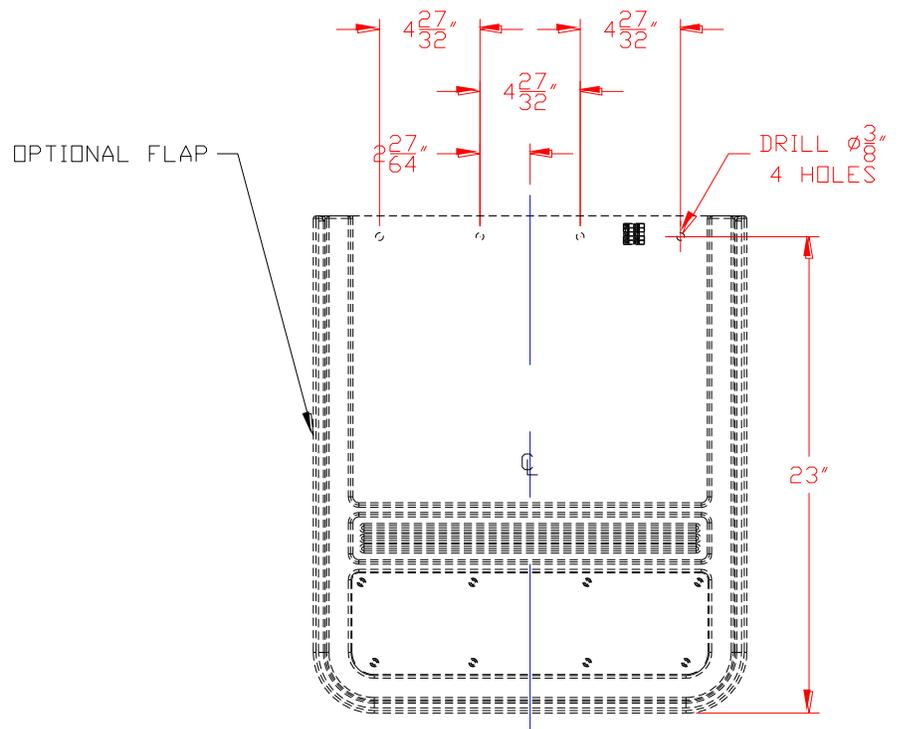
4. Assemble optional mud flap, mud flap bracket, pressure plate and rear strip with four carriage bolts, four 3/8" flat washers, four 3/8" lock washers and four 3/8" hex nuts (See diagram #3).
