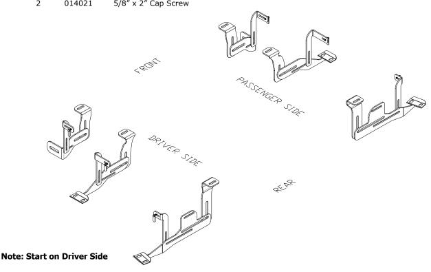
**Step 1:** Remove front cab mount bolt and install pre-assembled bracket loosely with the factory bolt. Watch out for bracket orientation. Set up the front bracket support strap using #762236 T-Bolt with #018046 3/8" flat washer, #024006 3/8" lock washer and #025015 3/8" hex nut.
