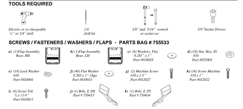
Prior to installation of your Mud Flap, see the above diagrams and parts list for all necessary parts.
