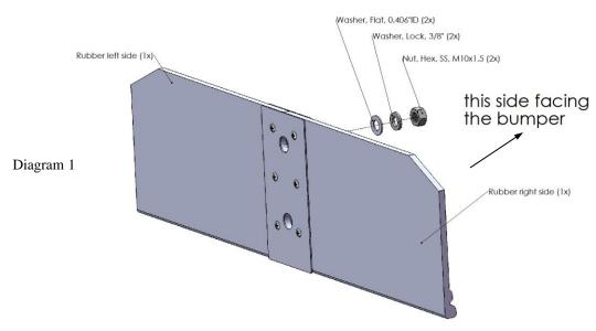
Position Guard between Bumper and Frame. Place the assembled Guard at the two OEM Factory Bolts (do not remove the existing OEM nuts, place guard in front of the OEM nuts), which are holding the frame for the Bumper. See pic 1. Install guard with washer/lock washer/hex nut and tighten them up.
