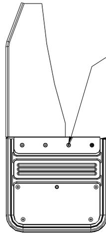
DRILL FOUR  $\varnothing 3/16"$  HOLES FROM THE STAINLESS PANEL THROUGH THE RUBBER FLAP
