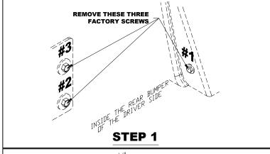
Step 1: Remove the three factory screws on holes #1 to #3.
