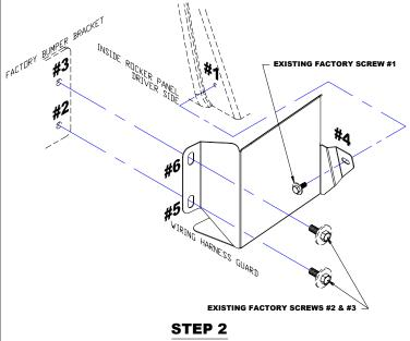
Step 2: Loosely install factory screw through guard hole #4 into factory hole #1, then install factory screws through guard holes #5 & #6 into factory holes #2 & #3.
