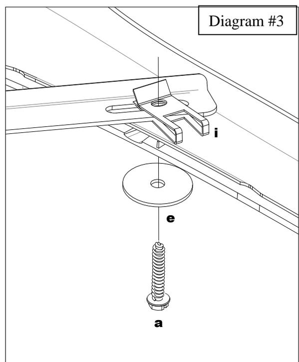
13. Install newly drilled mud flap holes # and # to bracket holes # & # using a sheet metal screw (a) and flat washer (e).
