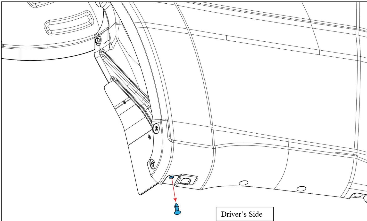
1-1 Remove factory push pin as shown
