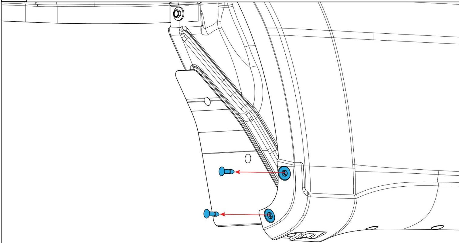
1-2 Remove factory push pins from fender as shown
