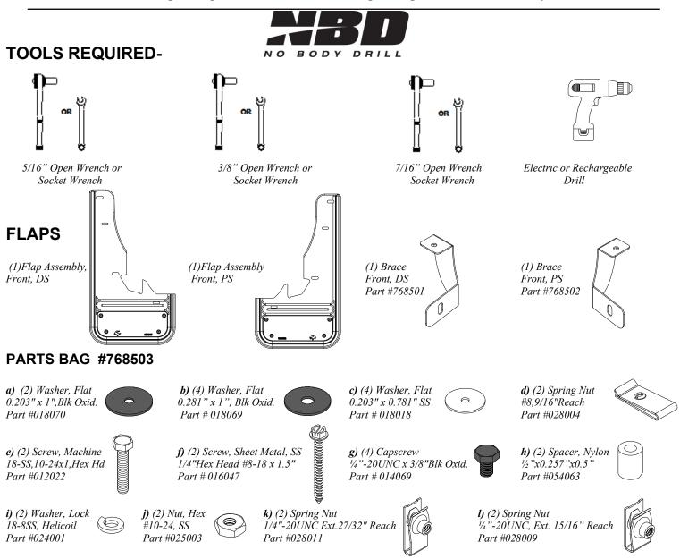
**INSTALLATION** (For ease of installation it is suggested that the wheel be removed)
