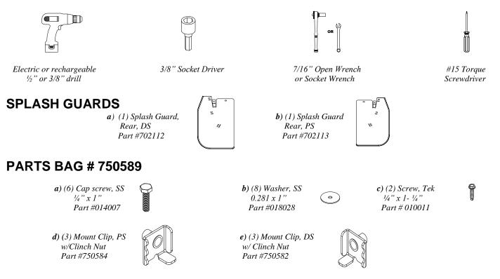
**INSTALLATION** (For ease of installation, it is suggested that the wheel be removed)
