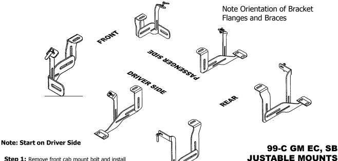
**Step 1:** Remove front cab mount bolt and install pre-assembled bracket loosely with the factory bolt. Watch out for bracket orientation. Set up the front bracket support strap using #762236 T-Bolt with #018046 3/8" flat washer, #024006 3/8" lock washer and #025015 3/8" hex nut.
