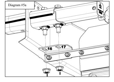
7b. For vehicles without crash bar, loosely install the mounting bracket through holes #16 & #17 to the factory crash bar mount holes #18 & #19 using an M12 bolt (k). (See Diagram #5b)
