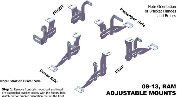
**Step 1:** Remove front cab mount bolt and install pre-assembled bracket loosely with the factory bolt. Watch out for bracket orientation. Set up the front bracket support strap using #762236 T-Bolt with #018046 3/8" flat washer, #024006 3/8" lock washer and #025015 3/8" hex nut.
