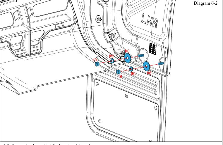
6-2: Secure hardware installed in step 6-1 as shown.
