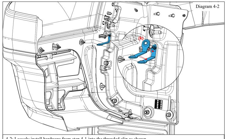
4-2: Loosely install hardware from step 4-1 into the threaded clip as shown.
