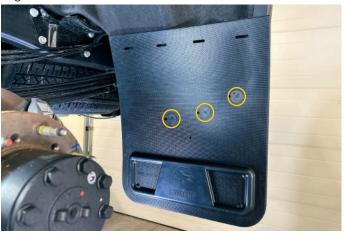
9. Hold rubber against the liner & mark the 2 upper left holes with a marker.
