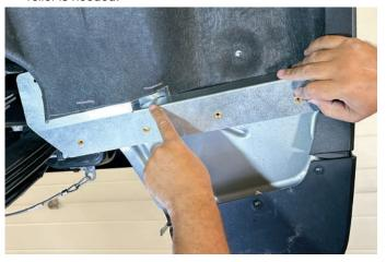
22. Mark the liner further, going slowly so that you aren't taking off more than you need. The objective is to be able to mount the bracket but leave enough of the liner intact so that it isn't visible once the mudflaps are installed.
