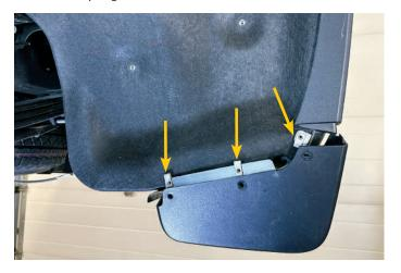
2. Pull the factory protector down so the spring nuts on the liner are exposed.
