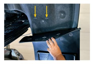
12. Roughly line up to 2 left lower holes of the bracket with the marks made & mark below the bracket with a marker.
