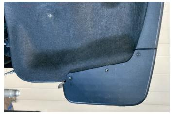
7. Loosely install mudflap using 3 factory holes in order to make guide marks.
